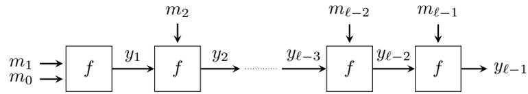
Figure 4: Merkle-Damgård hash mode processing  $\ell$  block messages with  $(\ell - 1)$  2-to-1 compression function calls
