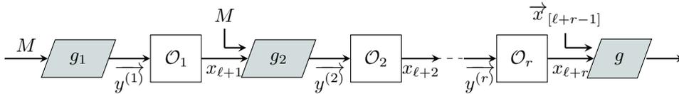
Figure 1: General Hash mode with  $\ell$  message blocks based on  $r$  calls to underlying  $t$ -to-1 oracles.
