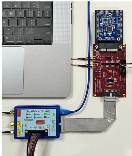
**Fig. 1.** ChipWhisperer-Husky, CW313 adapter board and CW308T-STM32F4 board used in the experiments.
